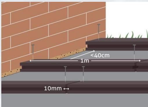
Allow a gap of at least 8mm between the end of the subframe and a fixed object such as a wall and at least 10mm gap on the subframe joins. This allows for proper drainage and temperature expansion.
