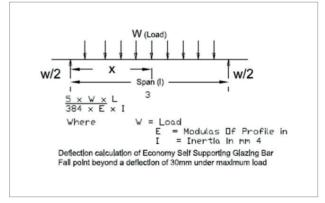
The Self Support Economy Glazing Bar is supported both ends with a  $622 n/m^2$  uniform load. The bar deflection is calculated at the centre of the roof.
