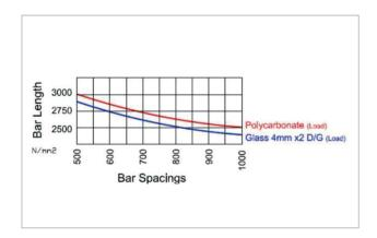
Deflection is calculated with a uniform load of 60Kg/m<sup>2</sup>.
